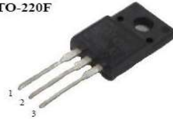
1. Gate 2. Drain 3. Source
